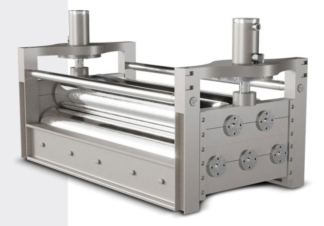
Usually on the entry part of pickling lines, composed of 4 pinch rolls and 5 straightening rolls.
