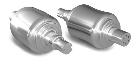
Manufactured from tool steel grades, induction or through hardened, used to straighten round bars and profiles.
